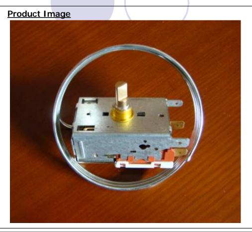
Usage: use in double door refrigerator and multiple door refrigerator Control temp. range:-30 ~ +10 Rating voltage:AC220V/AC110V, Rating current:5A,
